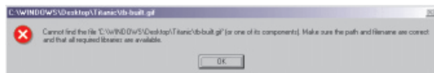
► Figure 3: If you don't delete the ddeexec sub-tree which was put there by Microsoft, applications such as Paint Shop Pro will get rather upset when you double-click GIF files, for example.
